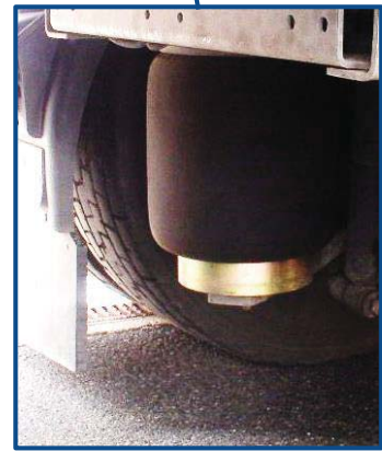
Gas accumulator example of an « Air ride » (pneumatic) suspension
