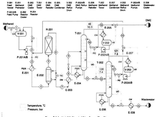
Figure 8.1.1 Unit 200: Dimethyl Ether Process Flow Diagram
