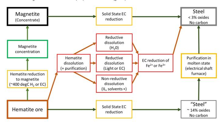
Flow diagram for dissolved iron (red) and solid-state (green) routes of iron ore reduction
